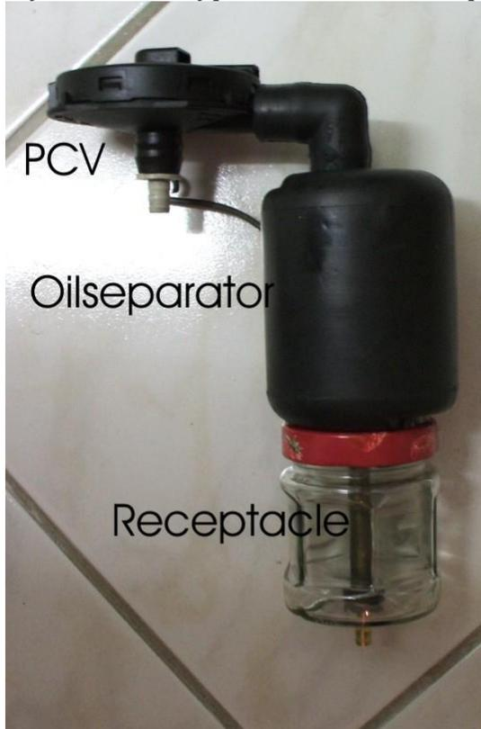
In an attempt to combine all the requirements in one device I therefore opted for a water-oil separator for a compressor also because it has a plastic receptacle so that you can see what is happening and it includes a tap for emptying the separator.
