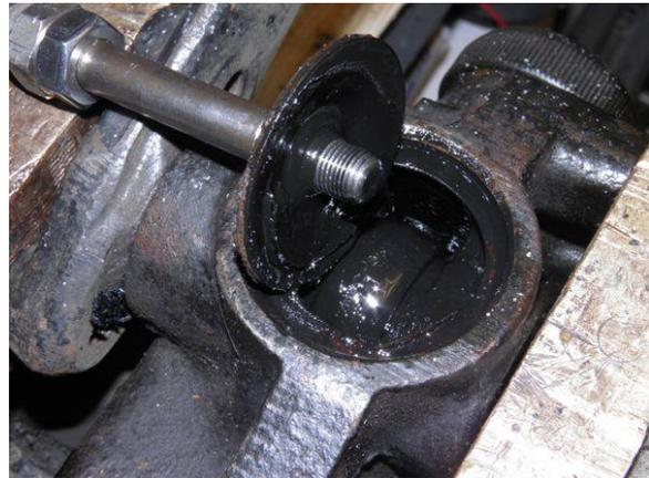
This success made me decide to use the same procedure for the metal disk opposing the damper arm rod end. It was found that the material of the disk is sufficiently thick to be able to cut a 1/8" BSP thread into a hole drilled at the center of the disk and by using the same threaded bolt the metal disk came out easily without any damage.
