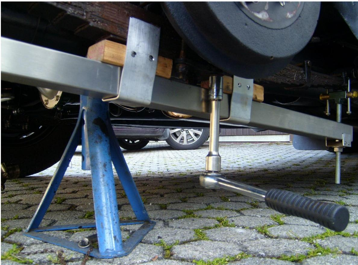
The supporting wooden blocks for contacting the middle of the spring are slidable and can so be adjusted to leave enough room for access to the nuts for the U-bolts.
